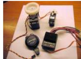
Hitec Segelwinde HS-785 HB - Graupner Servo C 577 - Hype Fahrregler Smart Control 20
